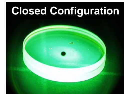
Two-disc penetrant sandwich effectively removing air interaction
